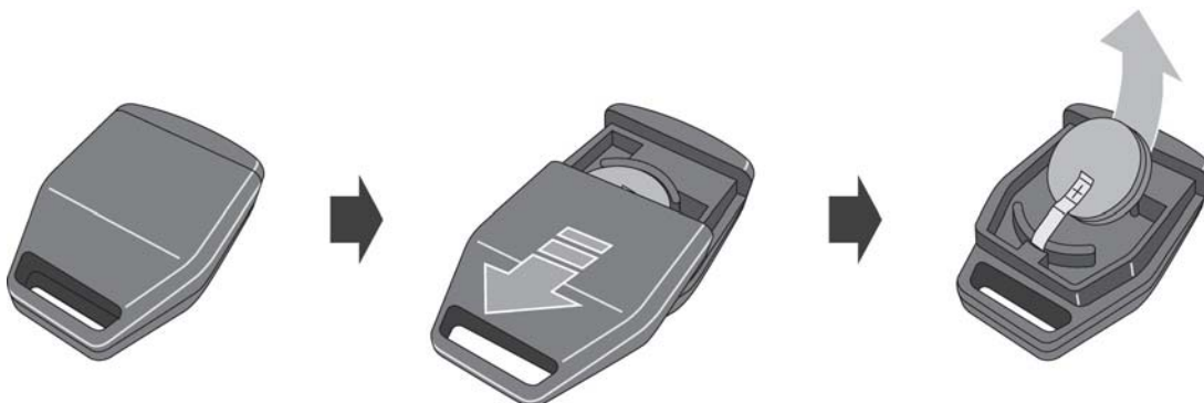
Fig. 5: Replacing the batteries in infra-red access keys
