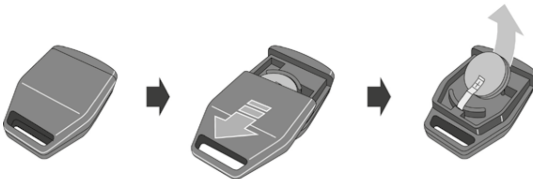
Fig. 6: Replacing the batteries in infra-red access keys
