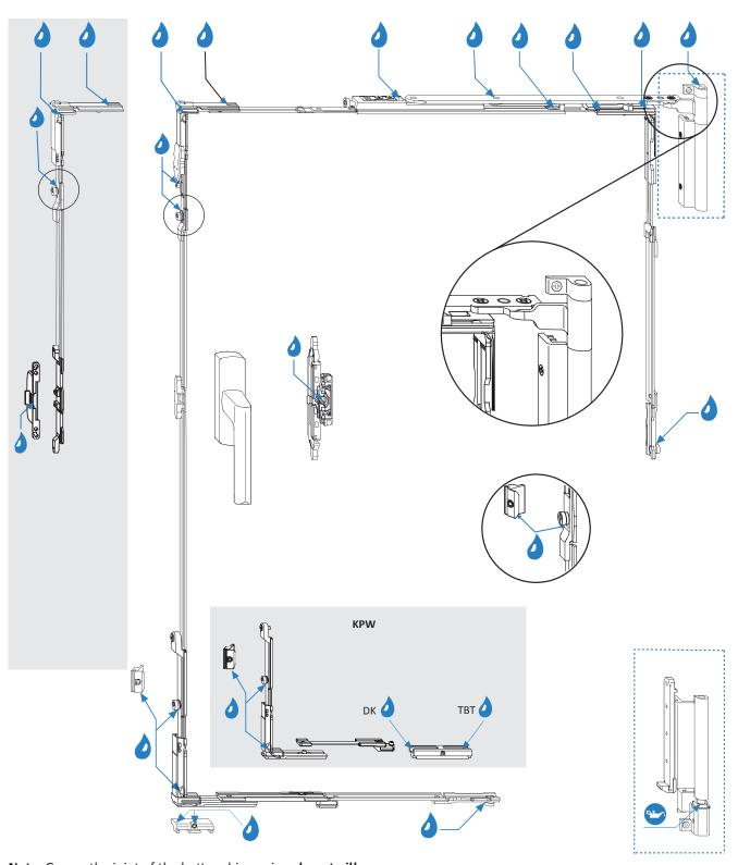
Note: Grease the joint of the bottom hinge pins, do not oil!
