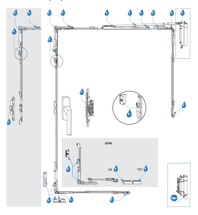
**Note:** Grease the joint of the bottom hinge pins, **do not oil!**
