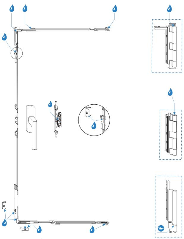
Note: Grease the joint of the bottom hinge pin, do not oil!
