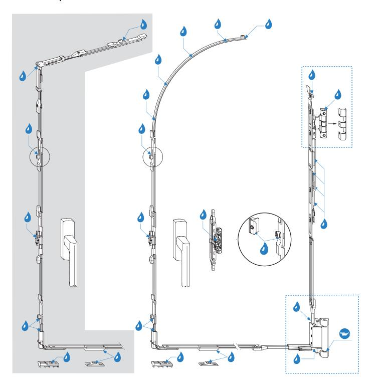
**Note:** Grease the joint of the bottom hinge pins, **do not oil!**
