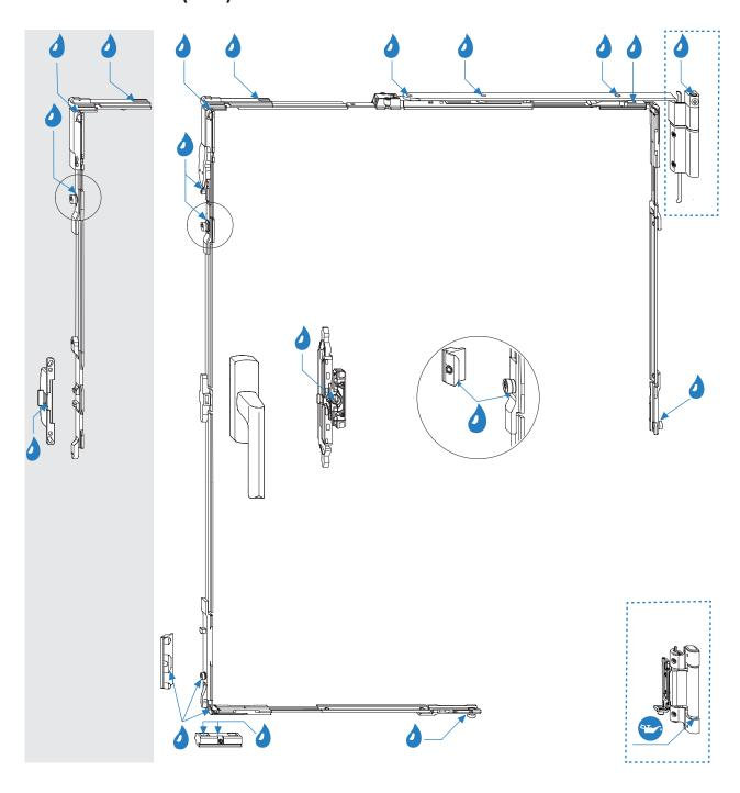
Note: Grease the joint of the bottom hinge pins,  $\operatorname{\textbf{do}}$   $\operatorname{\textbf{not}}$   $\operatorname{\textbf{oil!}}$
